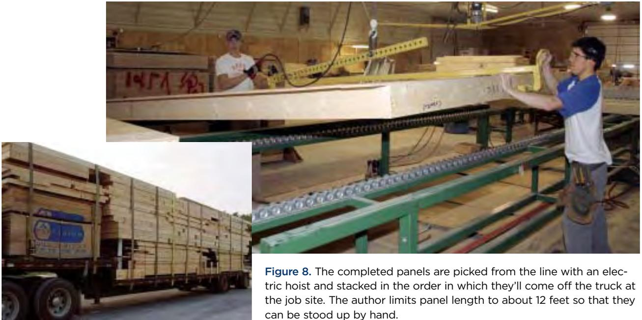
**Figure 8.** The completed panels are picked from the line with an electric hoist and stacked in the order in which they'll come off the truck at the job site. The author limits panel length to about 12 feet so that they can be stood up by hand.
