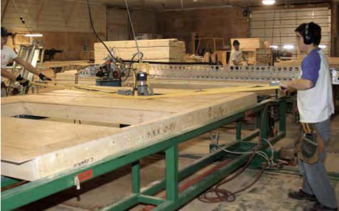
**Figure 6.** Window and door openings are cut with a 3<sup>1</sup>/<sub>4</sub>-hp router mounted on a steel sled. Suspended from a cable, it retracts out of the way when not in use and can cut out a door or window in about a minute.
